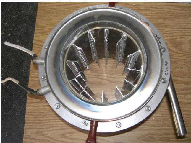
Fig. 3. Heat-conducting fins on converter inner wall to enhance heat transfer from gaseous combustion products to thermoelectric module.
